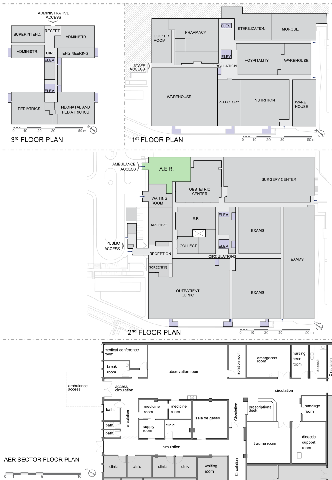
Illustration 5 . Schematic plans of the 1st, 2nd and 3rd floors, AER plan. Source: adapted from the archives provided by SEF HU-USP.
