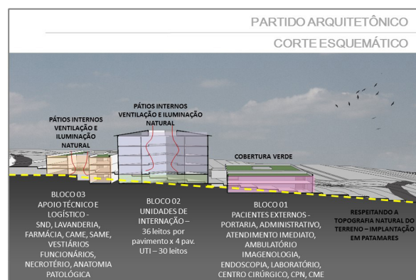
Picture 10 – Case 3 – Hospital Master Plan for a new hospital – Architectonic Project Simplified Plan. Source: Badermann Arquitetos, 2016.
