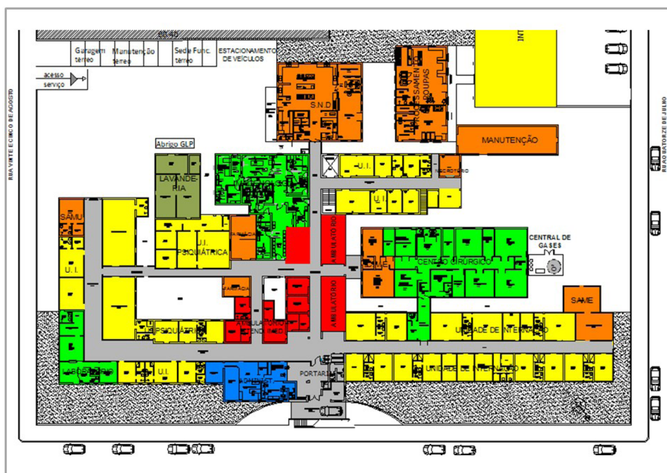
Picture 1 – Case 1 – Hospital Master Plan for an existing hospital – Floor plan with the existing zoning of the functional unities. Source: Badermann Arquitetos, 2015.
